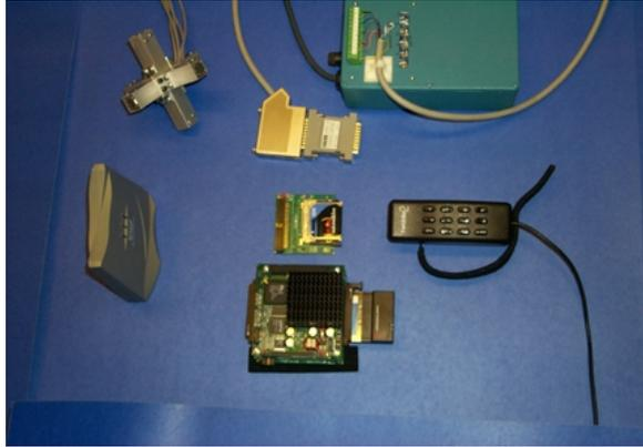
Figure 4. Components of the inertial tracker. The cross-shaped device in the upper left is the inertial tracker. The microprocessor (lower center) is worn by the user, and broadcasts tracking data offboard to the base station (lower left).
