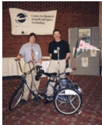
Figure 1: The Virtual Reality Tricycle. The VR Trike permits different combinations of visual and non-visual cues to be presented to an operator, but uses a HMD to generate the visual cues.
