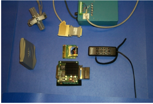
Figure 4. Components of the inertial tracker. The cross-shaped device in the upper left is the inertial tracker. The microprocessor (lower center) is worn by the user, and broadcasts tracking data offboard to the base station (lower left).
