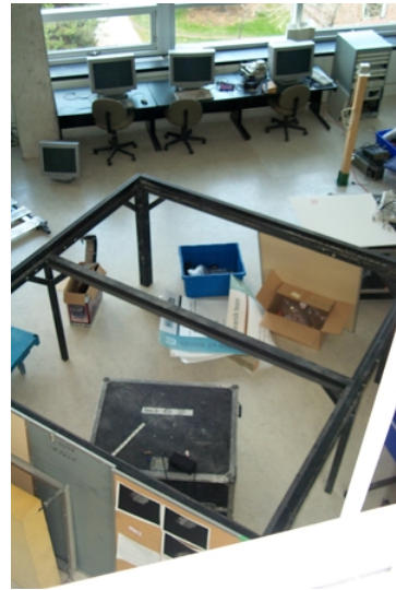
(b) View of the floor support taken from the 2 nd story of the VGR lab. A catwalk around the space provides access to the projectors and mirrors. Note that IVY's floor is located 4' above the physical floor of the lab.
