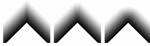
Image 3 - Artefacts caused by Gouraud Shading
