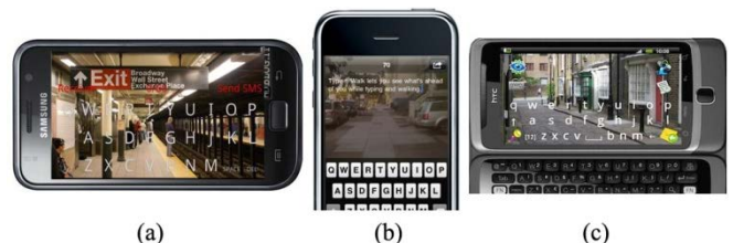
Figure 2. Recent commercial applications providing visual feedback via translucent virtual keyboard and/or text area: (a) Road SMS, (b) Type n Walk, and (c) Walk and Text.
