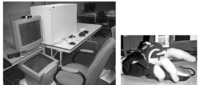
Figure 1. (Left) The experimental setup. The table to the right of the system was used for the horizontal support condition, and the cupboard resting on top for the vertical support condition. The table was removed for the unsupported conditions. (Right) Hand tracker and mouse – fingers lifted to show mouse underneath.
