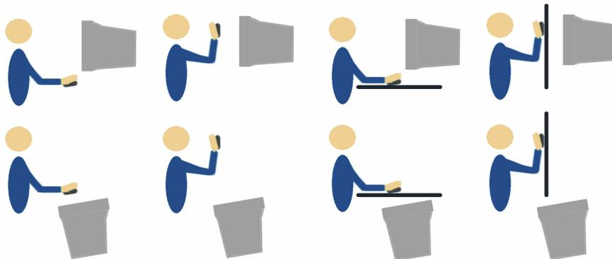
Figure 3. The eight experimental conditions. The left four represent the unsupported conditions, and the right four the supported conditions. The top four represent the vertical display, and the bottom four represent the horizontal display.
