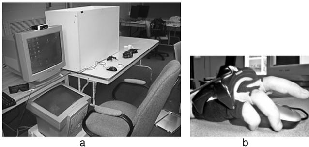
Figure 1. a) The experimental setup. The table to the right of the displays was used for the horizontal support condition, and the cupboard resting on top for the vertical support condition. The whole table was removed in the no support condition. b) Hand tracker and mouse – two fingers lifted to show mouse underneath.
