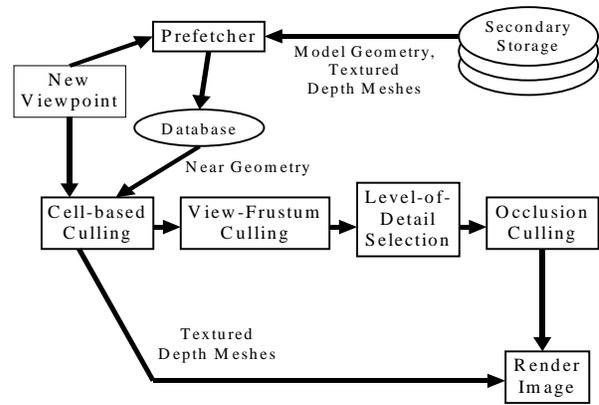
**Figure 1.** System Pipeline. Each new viewpoint sent into the pipeline is passed both to the prefetcher and to the rendering pipeline. The viewpoint determines what geometry and TDMs are retrieved from disk; it is also a parameter used by the rendering acceleration techniques.
