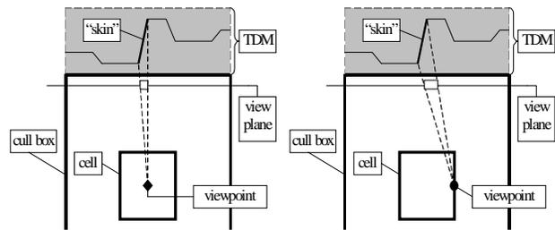
**Figure 3.** TDM Error Metric. (Left) Skin as seen from center of virtual cell. (Right) Skin as seen from the cell boundary. TDM error metric measures the maximum skin size, in screen-space pixels, for each cell.
