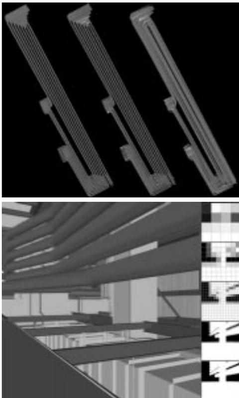
**Color Figure C.** Example Rendering Acceleration Methods: (top) LOD - multiple geometric levels of detail are computed for complex objects, (bottom) occlusion culling - the flooring, column, and a portion of the pipes function as occluders that allow the hidden geometry to be safely culled (a hierarchical set of occlusion maps are displayed on the right side of the screen).
