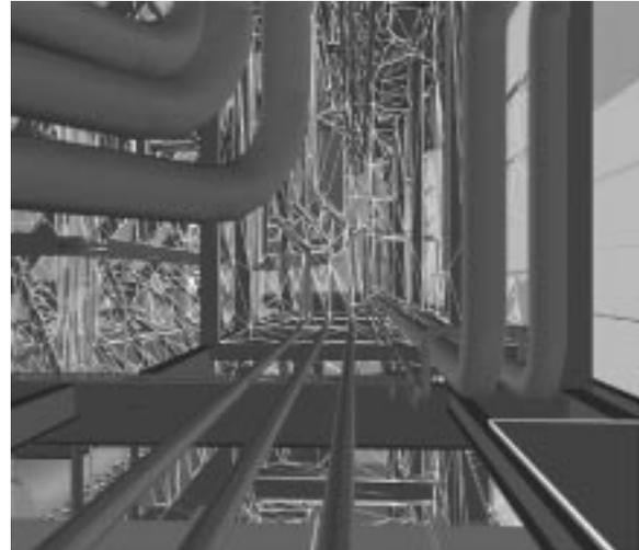
**Color Figure B.** Example TDM. Textured depth meshes replace distant geometry. Polygons outlined in white are part of a TDM. Near geometry is rendered conventionally.
