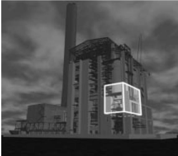
**Color Figure A.** Bird's eye view of a power plant model. We have outlined in white the subset of a power plant rendered as geometry for an example viewpoint inside a cull box (model courtesy of James Close and Combustion Engineering, Inc.). This geometry is rendered using levels of detail and occlusion culling. Darker colored geometry is replaced by a fast image-based representation.
