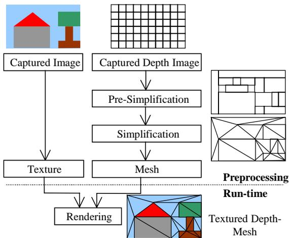
**Figure 2.** Offline and online components of textured-depth mesh generation. The preprocess generates a texture and a mesh from a captured image and a captured depth image; the textured depth meshes are displayed at run time.
