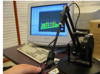
Figure 1. Virtual Lego System and Phantom Device.
