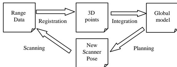
The four stages of the acquisition pipeline are iterated until the object is completely scanned.
