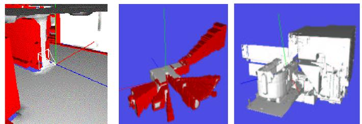
Integration and planning for an extremely large scene. The surface net algorithm allows fast surface extraction even for large models.
